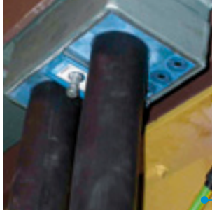
Driver's cabin: The Roxtec S 6x1 is used for mechanical anchorage of cables and reduced vibration.
